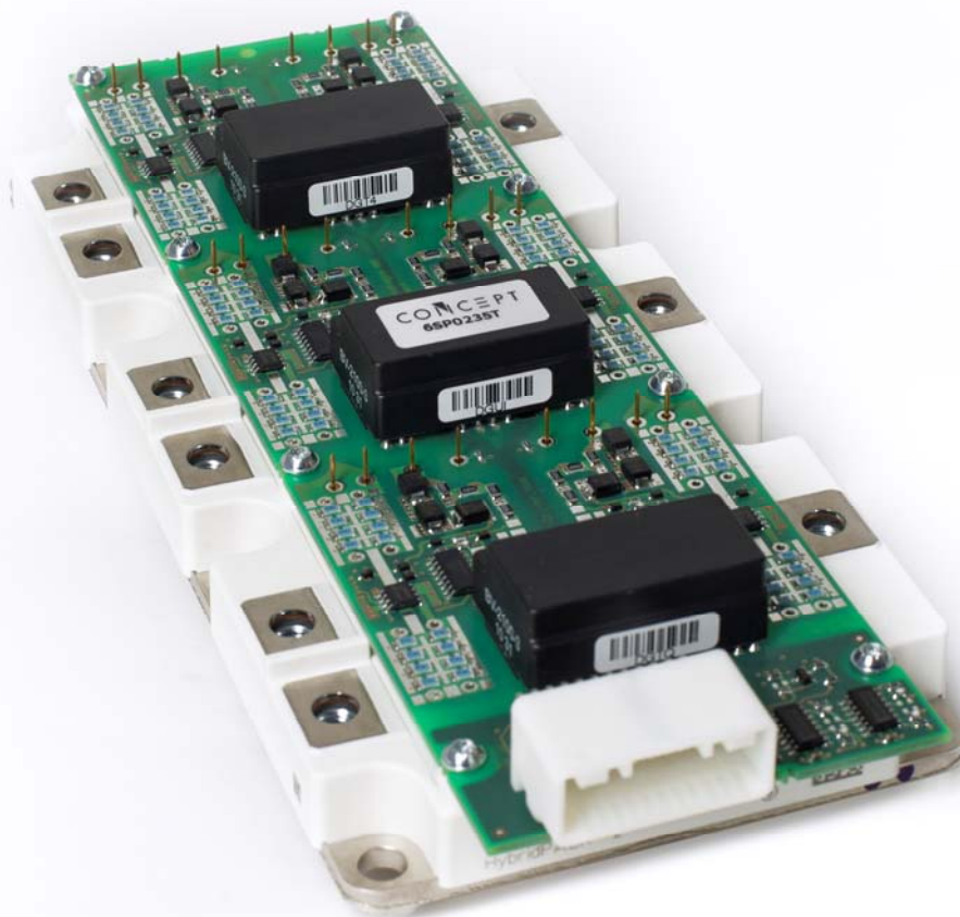
Fig. 1 6SP0235T soldered onto a HybridPACK™ 2 IGBT module
